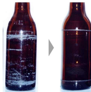
② Condition of abrasion on the body of the bottle The current bottle has limited whitening.
