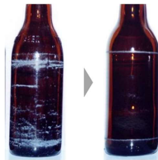
② Condition of abrasion on the body of the bottle The current bottle has a limited area of whitening.
